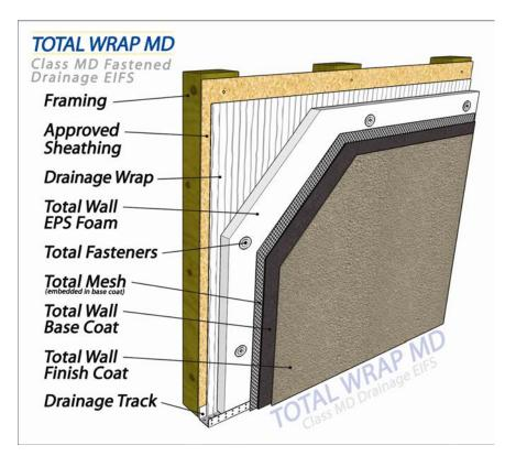
The **Total Wrap MD** system is a moisture drainable exterior wall cladding that utilizes a sheet applied moisture barrier plus a drainage plane as secondary protection against water intrusion.
