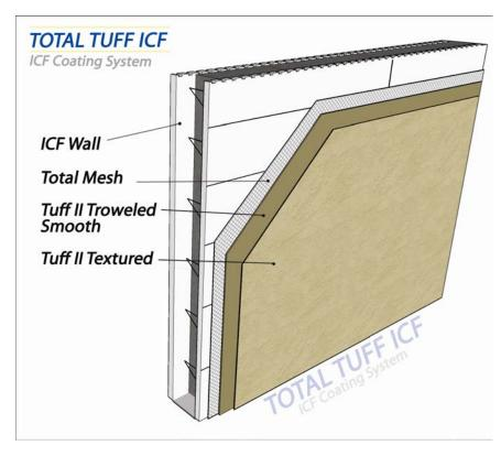
The **Total Tuff ICF** system utilizes our all in one base, primer and finish coat, Tuff II, embedded with our reinforcing mesh as the base coat. A second coat of Tuff II may also be used as the finish coat, or a standard Total Wall textured finish may be used.
