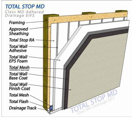
The **Total Stop MD** system is a moisture-drainable Class MD EIFS that utilizes Total Stop RA, a roller or spray applied liquid membrane as a moisture barrier with vertical ribbons of adhesive.
