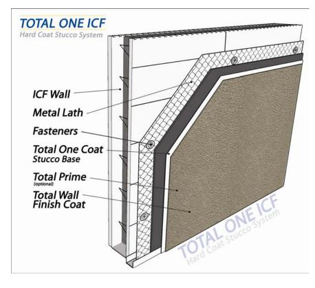
The **Total ONE ICF** system is traditional hard coat fiber-reinforced Portland cement stucco applied over Insulated Concrete Form (ICF) construction.
