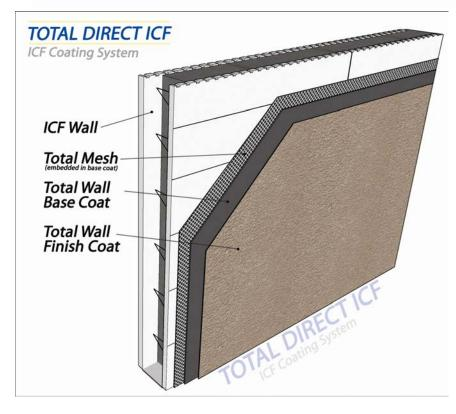
The **Total Direct ICF** system is a thin stucco veneer applied directly over an approved insulated concrete form construction.
