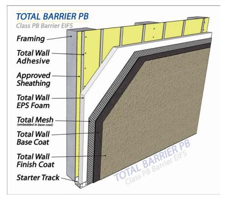
The **Total Barrier PB** system is a Soft Coat barrier Class PB Exterior Insulated and Finish System. It is suitable for use over non-moisture sensitive substrates.
